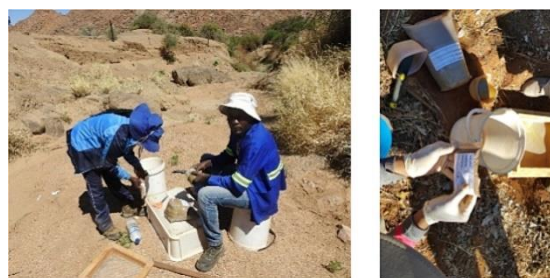
Figure 3. Sample collection from a drainage channel showing the two size fractions collected
