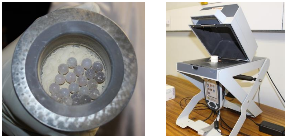
Figure 4. Sample preparation in an Agate Ball Mill (left) and analysis by Niton ED-XRF (right)
